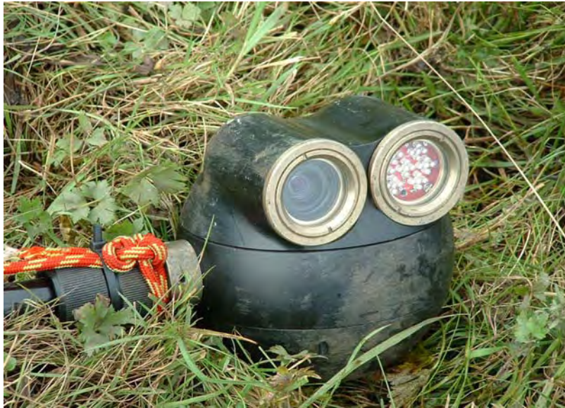
Figure 2 The Spyball camera with back-up rescue rope to retrieve the camera if the umbilical cable detaches
